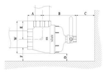
\*C – Clearance required for cap removal in case of maintenance.
